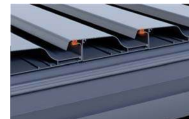
Multi-layered sealing system using several gaskets
